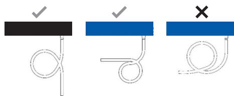
D) Fill the trap with water connect the hose to the unit outlet and secure it with a strap
