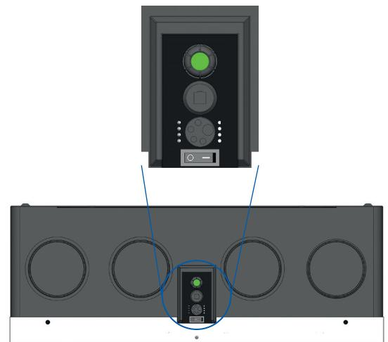
The two cable glands on the panel allow easy passage of the power and sensor cables and ensure the device is sealed.
