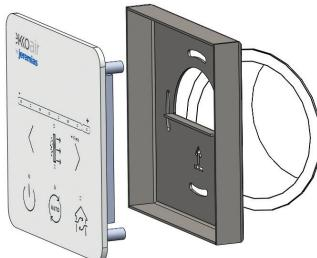
**D) Gehäuse an der Wand befestigen**
